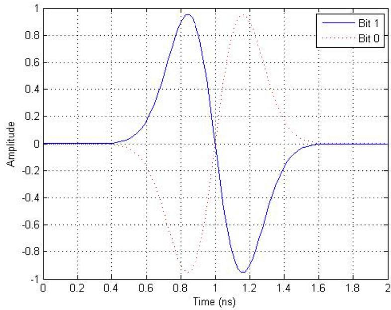
Figure 12. Binary PAM pulse shapes for "1" and "0" bits.
