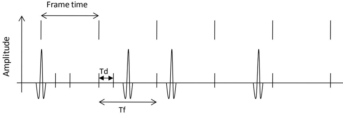
Figure 16. Four-ary PPM signal.
