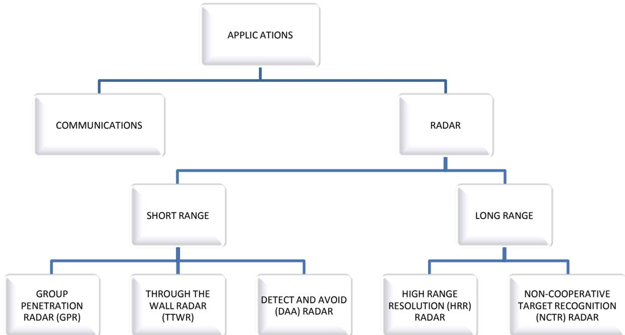
Figure 1. Ultra wideband applications in both communications and radar.
