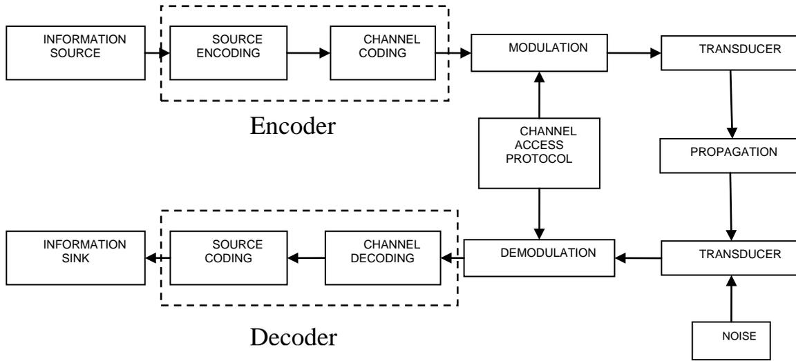
Figure 11 Generic architecture of a communication system.
