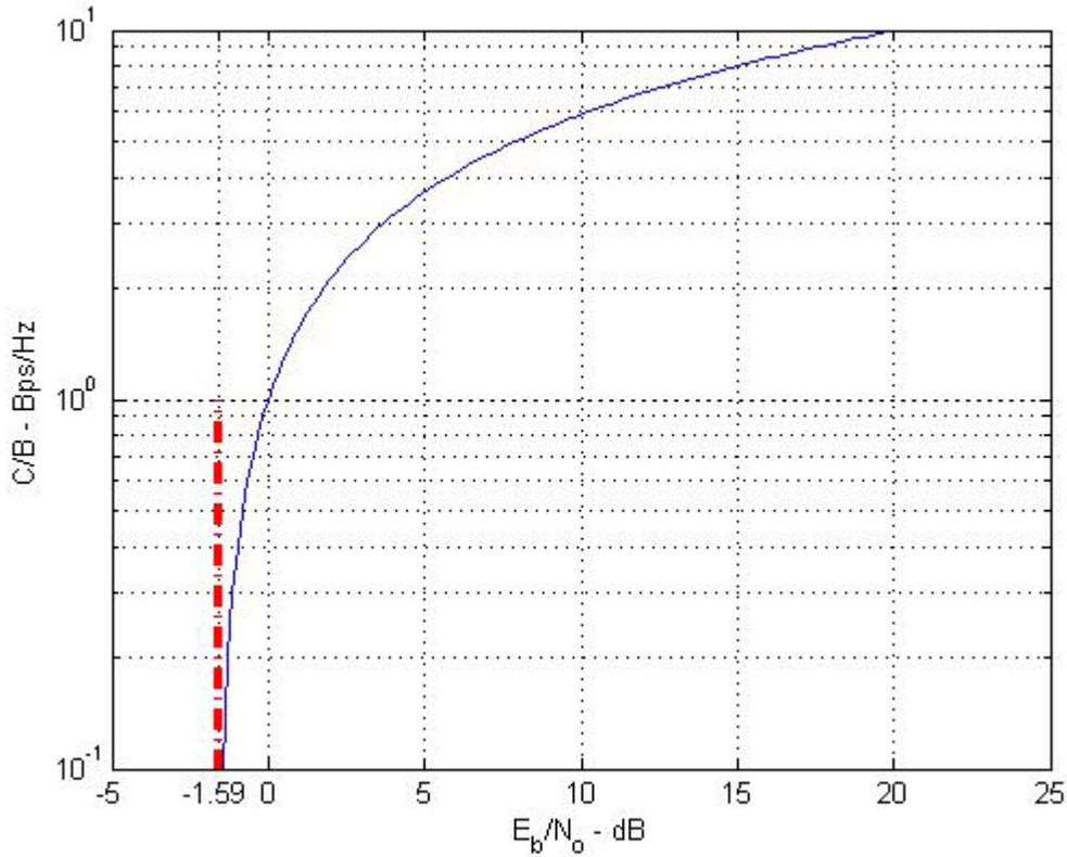
Figure 9. Communication efficiency limit: channel capacity/bandwidth ratio versus  $\frac{E_b}{N_o}$ .
