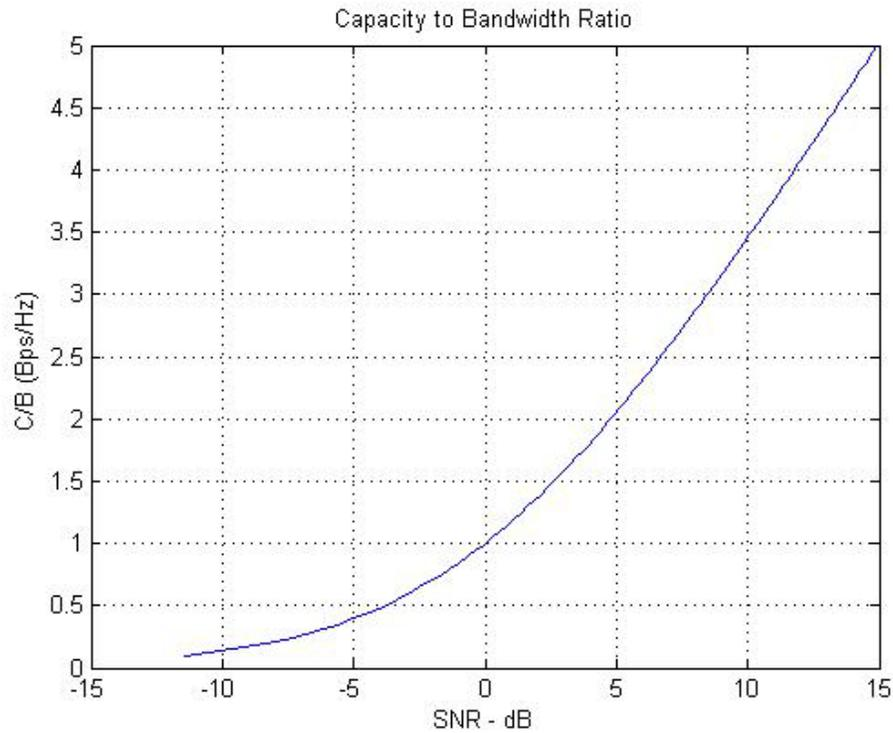
Figure 7. Ideal normalized channel capacity as a function of SNR for an AWGN channel.
