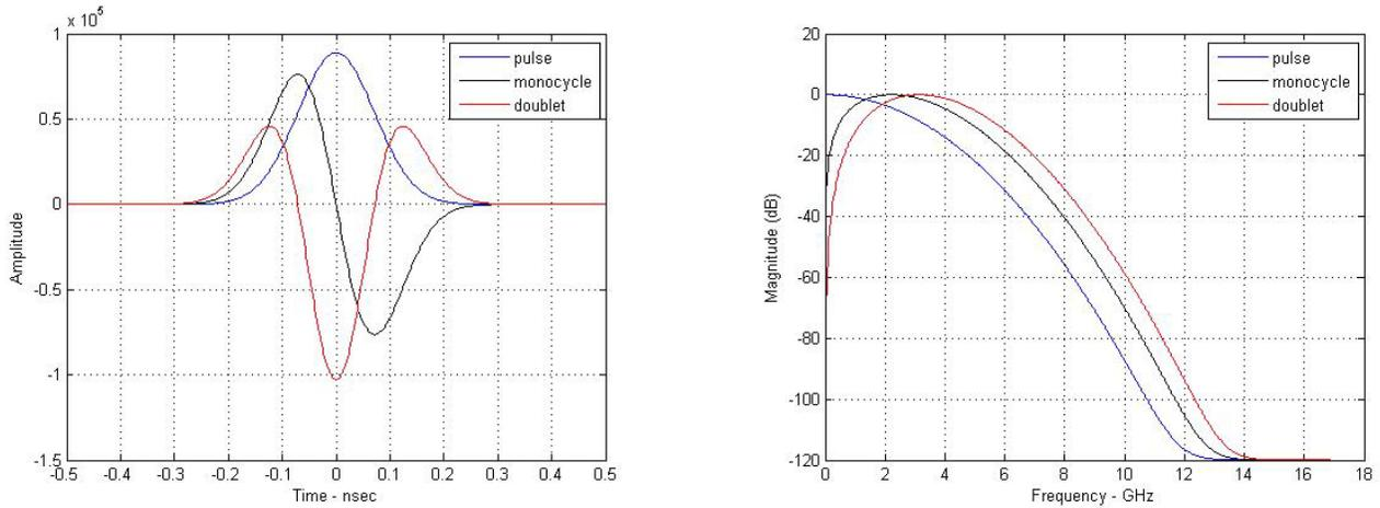
Figure 2. A Gaussian pulse, monocycle and doublet in the time and frequency domains.
