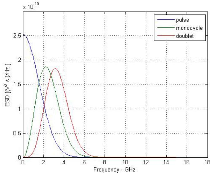
Figure 3. Energy spectral density for a Gaussian pulse, monocycle and doublet.
