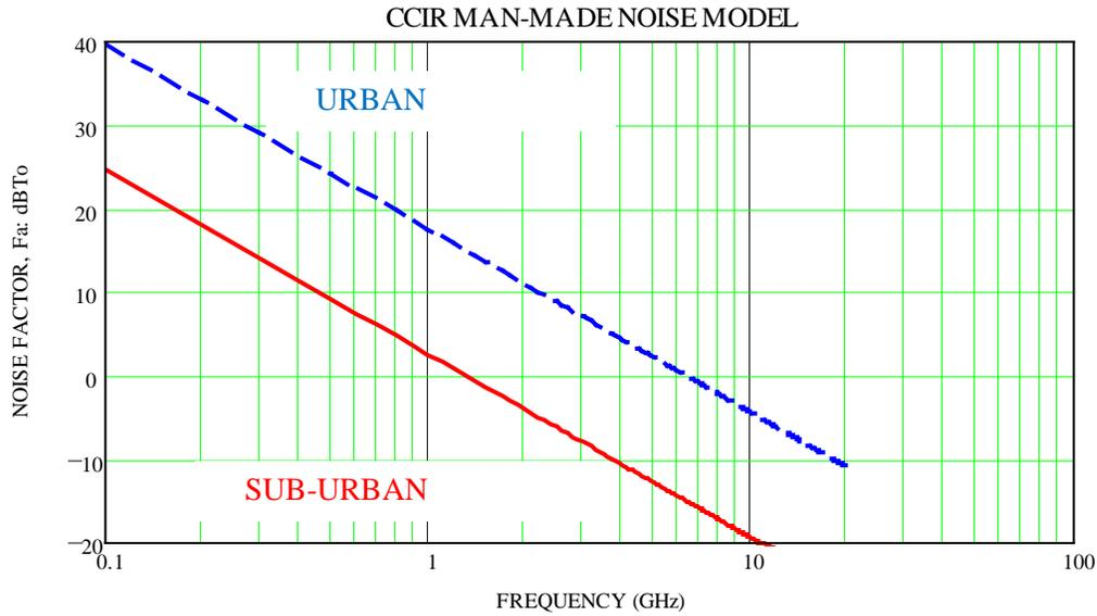
Figure 6. Man-made noise model.
